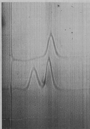
Figure 4. Sedimentation velocity patterns in 0.01 M phosphate buffer (pH 7.9): (lower) arachin; (upper) fraction corresponding to peak I in Figure 2B.
